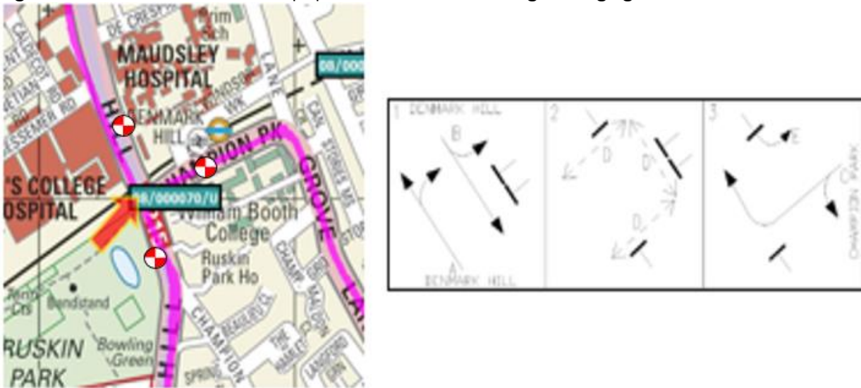
Figure 12 – J08/070 location map, position of VDPs and signal staging method of control
